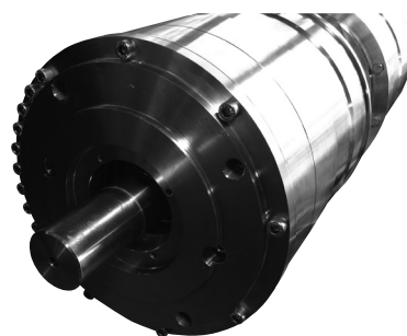
20. When the motor flange reaches the housing, the motor flange is on the right position. Mount the rest of the screws, replace the 3 M8x60 with normal screws and fasten all of them to 30 Nm \pm 3 Nm using the torque wrench.
