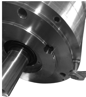
18. Screw the 3 M8x60 screws with nut in three treads so they are equally separated from each other. Torque the screws slightly and fasten the nuts until they make contact with the motor flange.
