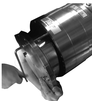
7. Remove the long M8x140 screw and the end flange. Warning: flange with swash plate is heavy, so make sure not to drop it. Risk of injury.
