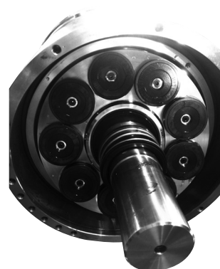
20. Remove the motor flange following the same steps described for the end flange (steps 2 to 9). Using the M8 x 140 mm is optional.
