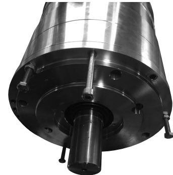
19. Fasten the 3 nuts one turn at a time to press the motor flange into the housing as straight forward as possible.
