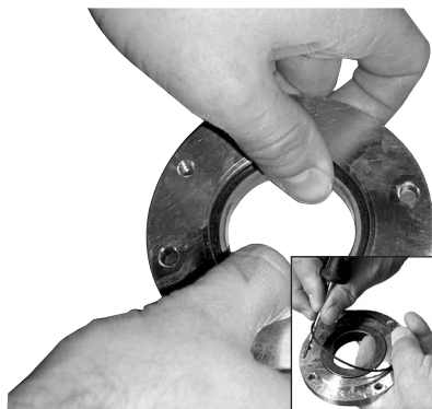
19. Remove ceramic ring from the cover for shaft seal by gently pushing it from the back of the sealing ring.
