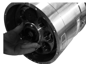
10. Remove by hand the pistons one by one. Be careful not to scratch the pistons. Tilt the retainer plate as needed for easy removal of pistons. When removing the last pistons, hold with one hand the retainer plate to make sure the retainer plate does not drop out. WARNING: Do not use any tools.
