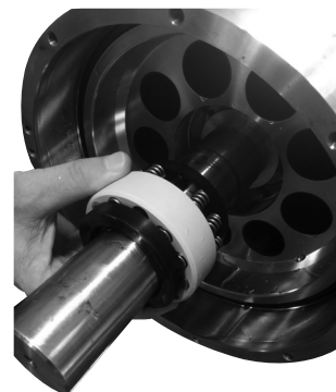
22. Remove pistons, retainer plate, retainer ball and spring package following the same steps described before for the end flange side (steps 10 to 13).
