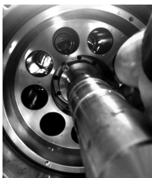
23. Mount 3 M10x15 in the valve plate through the holes in the cylinder barrel and fasten them with low torque. Be aware that only three holes in the valve plate have a thread.
